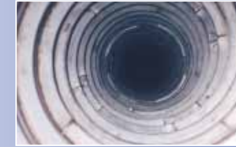
Internal spiral of a stainless steel dryer.
