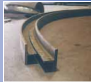
Angle rolling. Sizes up to 6" x 6" x 3/4" (160 x 160 x 20 mm).
