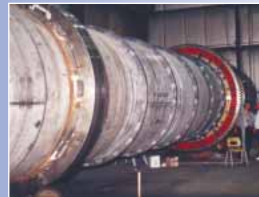
7'-5" Diameter x 55' Long Stainless Steel Dryer.
