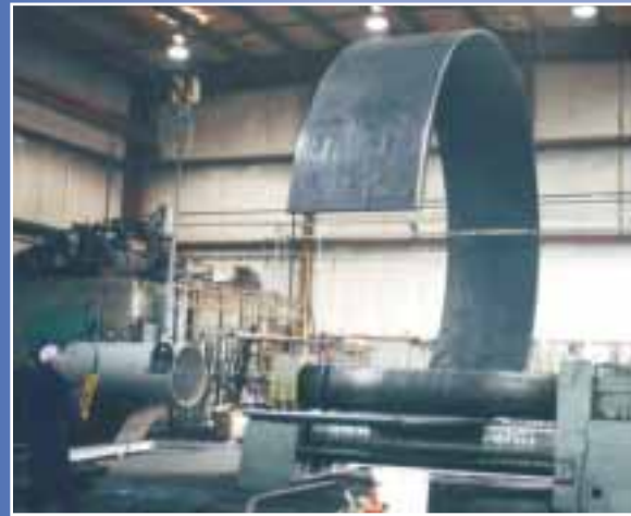
Rolling of heavy plates and sections. Sizes up to 120" (3 m) wide x 7 5/8" (195 mm) thick.
