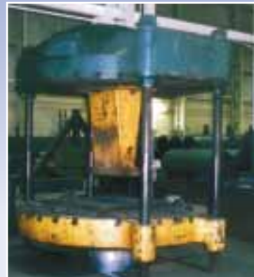
200 ton Four Post Press for straightening and repair of damaged and heat distorted weldments.
