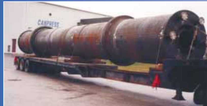
Process Drum, built complete with tires, gear, bearings, hoods and drive system.
