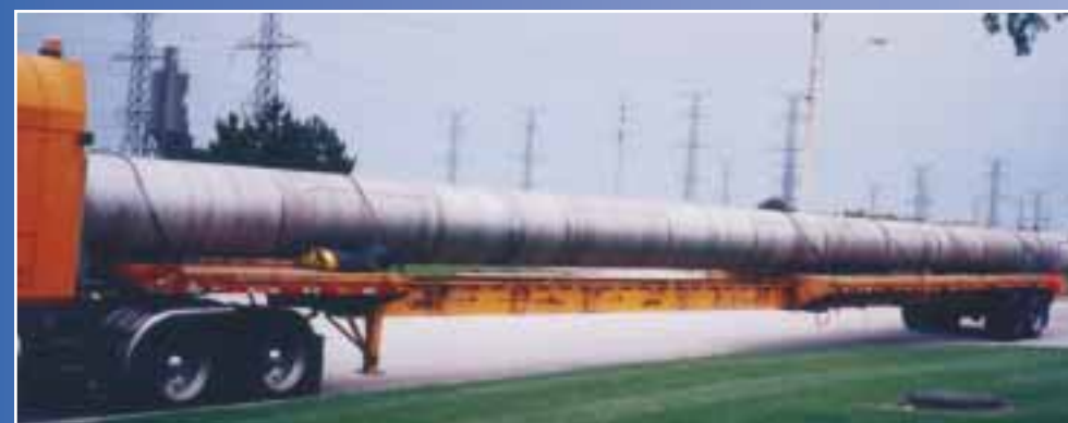
40" Diameter x 171' High Stainless Steel Stack for chemical plant.
