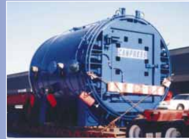
11' Diameter x 19' Long Explosion Containment Chamber for explosives research built completely by Canpress, including all operating mechanisms, hydraulics, controls and computer data acquisition.
