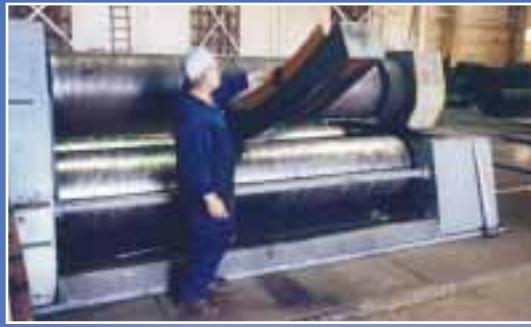
Rolling of heavy plates and sections. Sizes up to 120" (3 m) wide x 7 5/8" (195 mm) thick.
