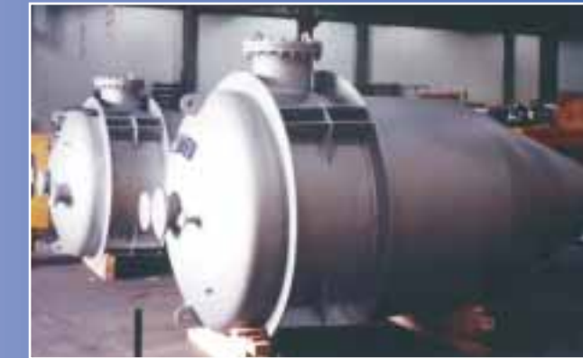
Product discharge Pressurized Bins for Iron Plant in Saudi Arabia. Designed for cyclic load pressure.
