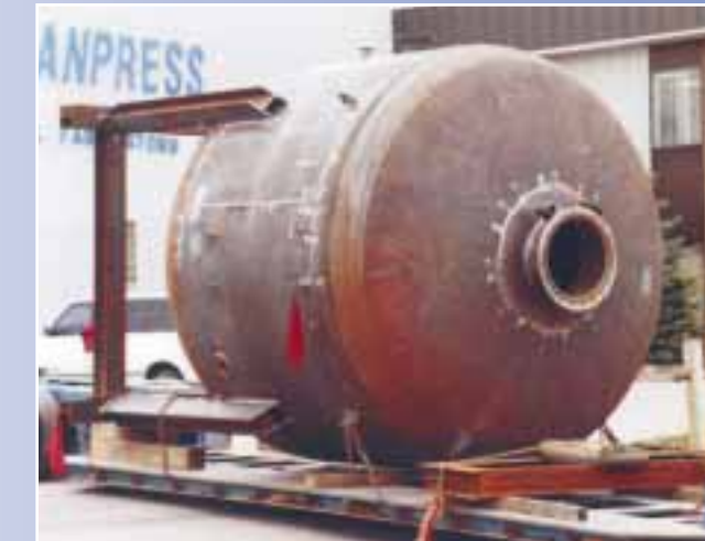
Water Treatment Tank 10' Diameter.
