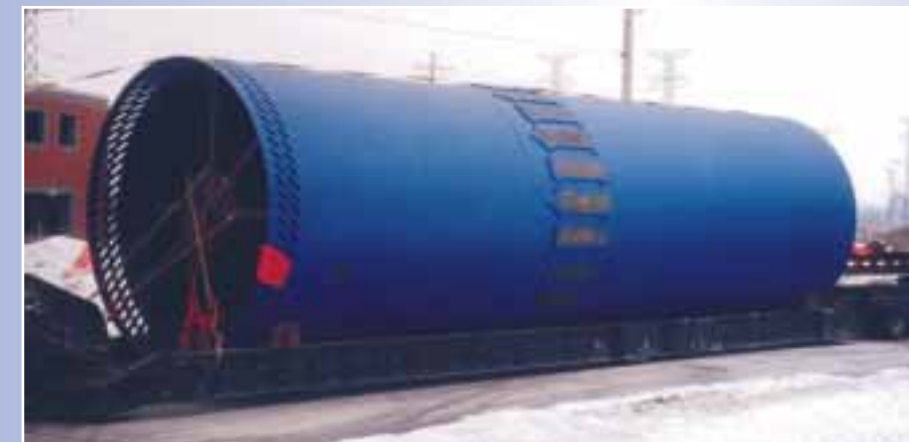
14' Diameter x 100' Long kiln shell section for fertilizer plant in New Mexico, USA.
