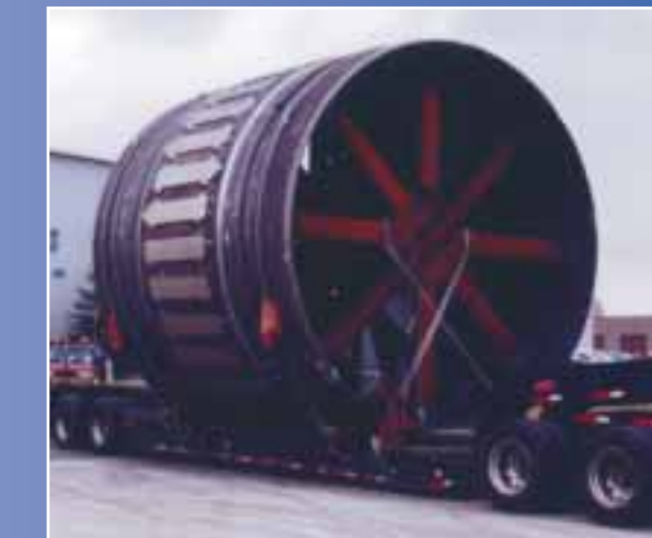
17'-9" Diameter kiln shell section.
